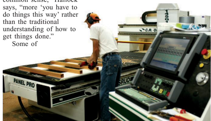
Jason Cooper operates the CNC machine, the high-tech component of drilling out the wood pieces of beds
